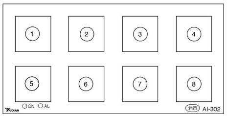
When D0 $\sim$ D7 is connected to COM terminal, the corresponding LED light  $1\sim$ 8 will flashing.
